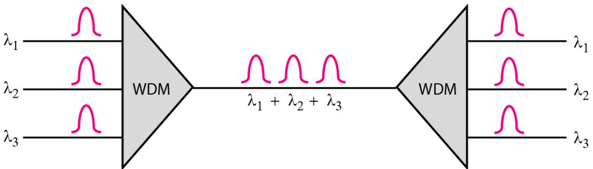
Using this technique, a multiplexer can be made to combine several input beams of light, each containing a narrow band of frequencies, into one output beam of a wider band of frequencies. A de-multiplexer can also be made to reverse the process.
