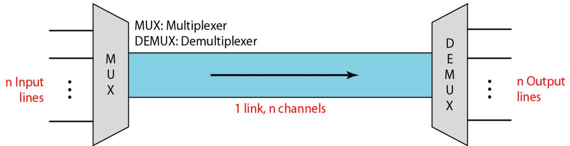
There are three basic multiplexing techniques: frequency-division multiplexing, wavelength-division multiplexing, and time-division multiplexing. The first two are techniques designed for analog signals, the third, for digital signals.
