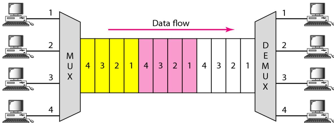
**We can divide TDM into two different schemes:** synchronous and statistical.
