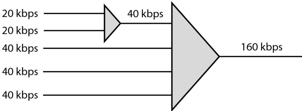
**2. Multiple-Slot Allocation** Sometimes it is more efficient to allot more than one slot in a frame to a single input line. For example, we might have an input line that has a data rate that is a multiple of another input. In Figure, the input line with a 50-kbps data rate can be given two slots in the output. We insert a serial-to-parallel converter in the line to make two inputs out of one.
