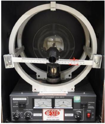
Figure 2: Experimental set-up for determining the specific charge of the electron
